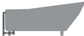
Exposed Bath Waste and Overflow
