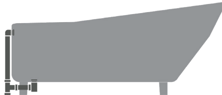
Exposed Bath Waste and Overflow
